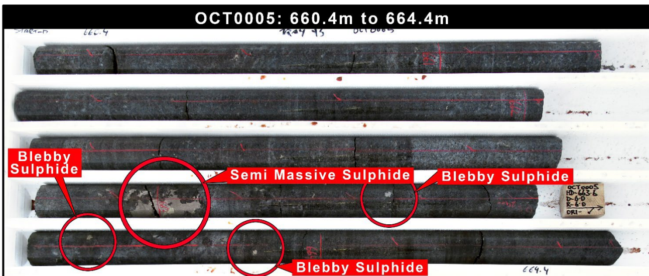
Photo 2: Diamond drill core tray from OCT0005 with visual Ni-Cu sulphide mineralisation. OCT0005 intersects the top edge of conductor 2 .
