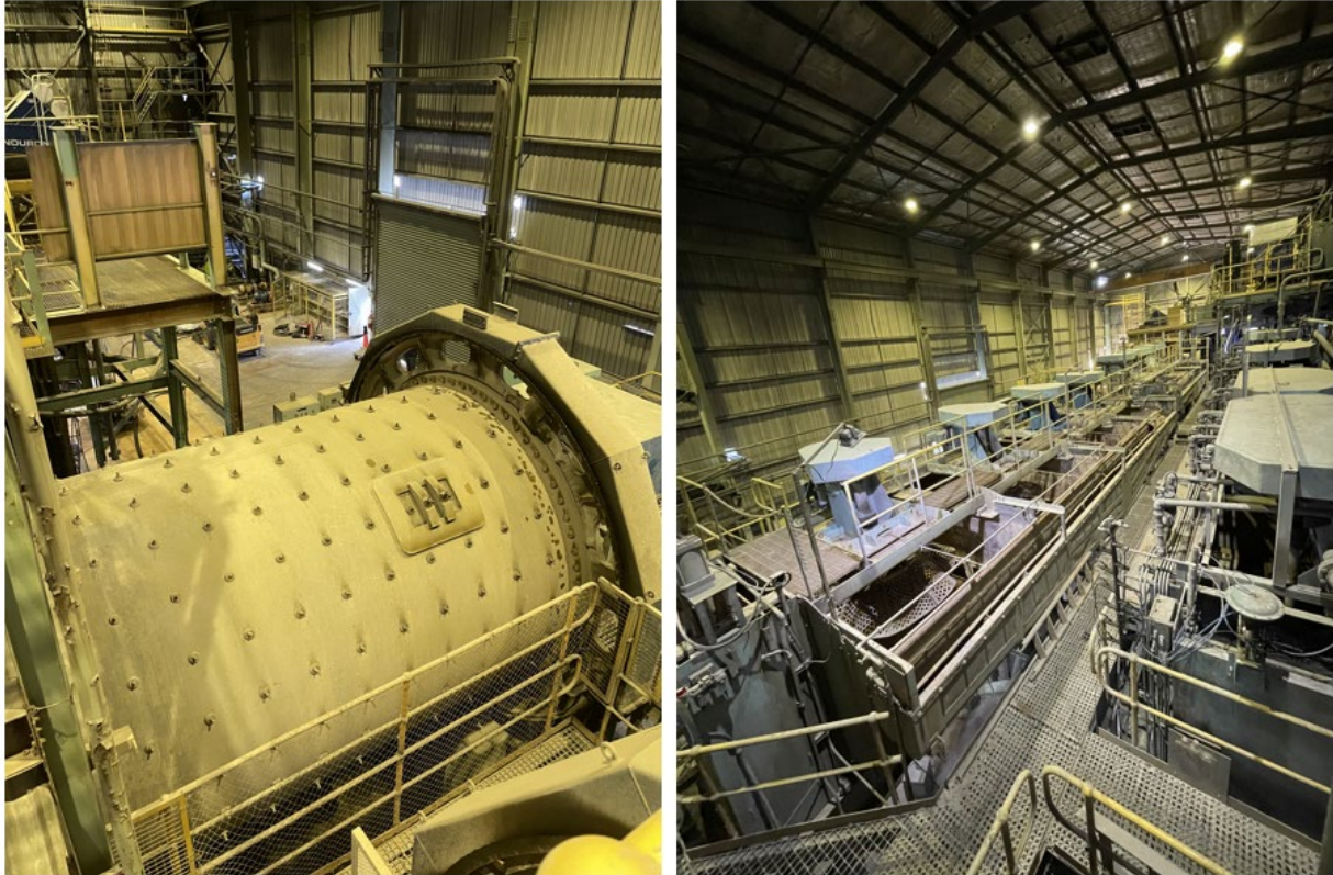
Figures 4 and 5: Ball mill and rougher/cleaner/scavenger units in mill.
