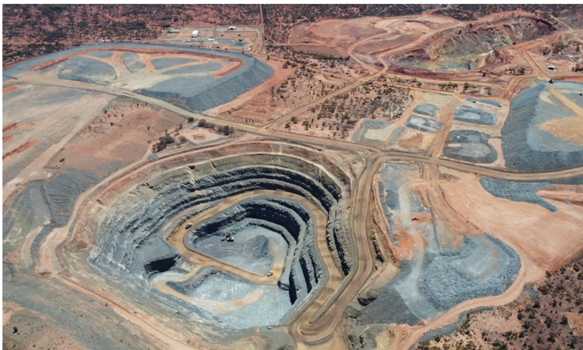
Figure 8 - Looking north over Missouri Open Pit to Sand King Open Pit and highlighting the reduced strip ratio in the Missouri Open Pit
