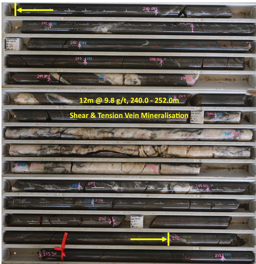
Figure 11 - SKD23004 Core from Sand King showing intersection of shear and tension veins
