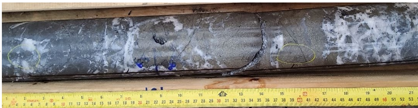
Plate 3. Drill hole PPDD23-001 semi-massive sulphide-quartz vein intersected at 88.57m
