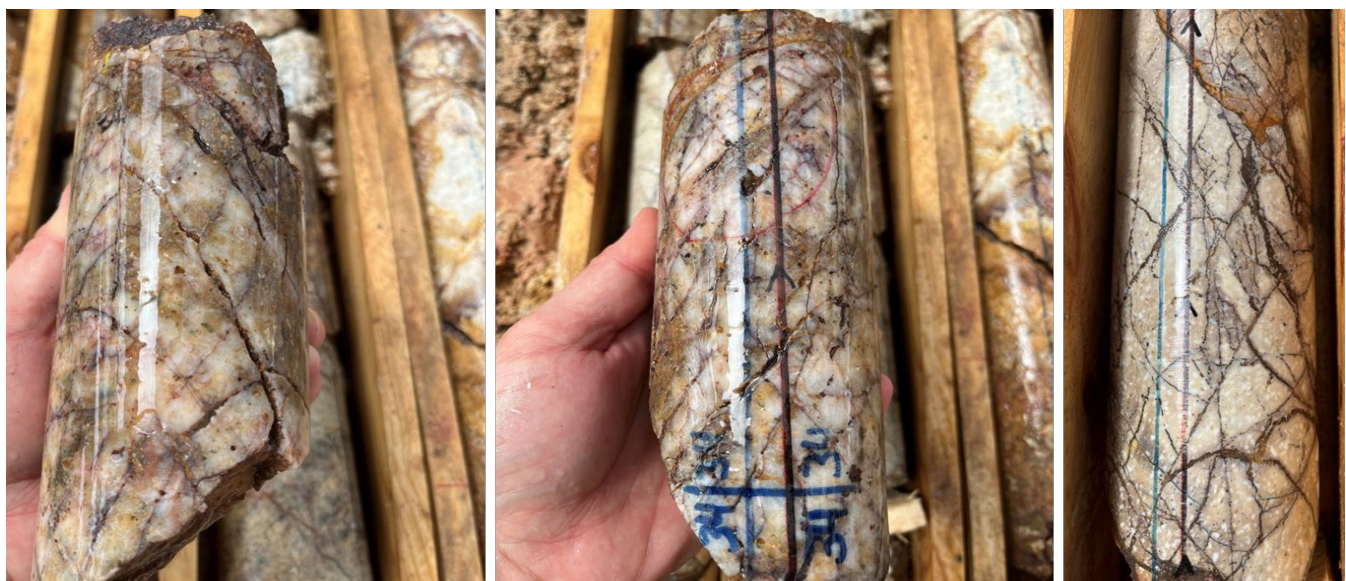
Plate 1: Drill hole PPDD23-002 displaying typical vein styles observed in diamond core between 22m and 39m at the Julia target.
