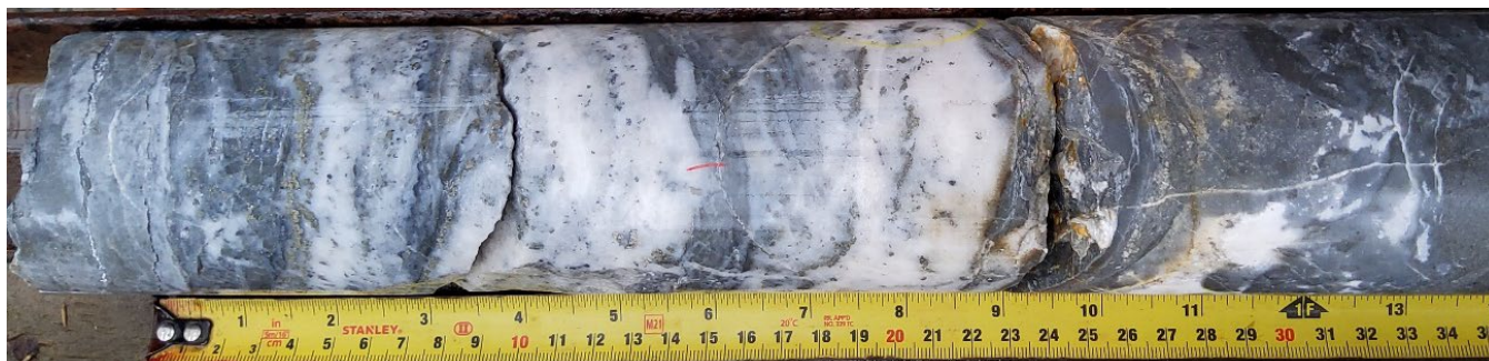
Plate 2: Drill hole PPDD23-001 epithermal vein intersected at 66.37m
