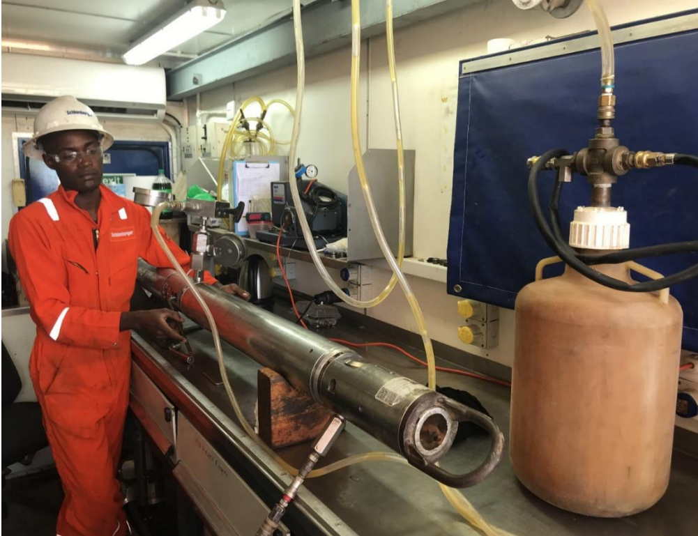
Figure 3 - Blowdown of Pebbly Arkose fluid sample where natural gas was recovered from a depth of 2197.3mMD
