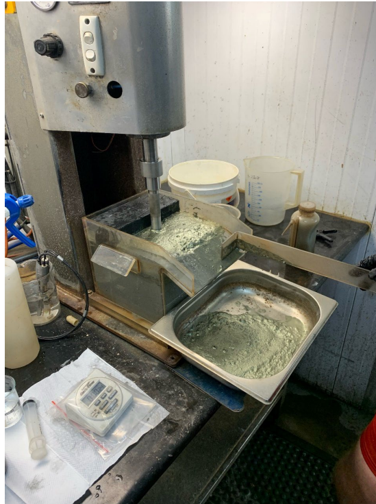
Concentrate collection during flotation testwork
