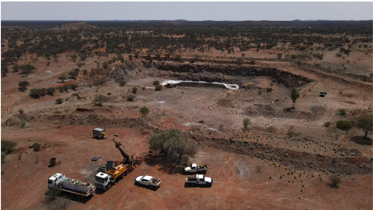
Figure 4: Aerial view looking SW showing the drill rig set up on first drill pad at Molyhil with the historically mined open pit in background.
