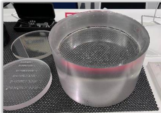
Sapphire blanks and boule
