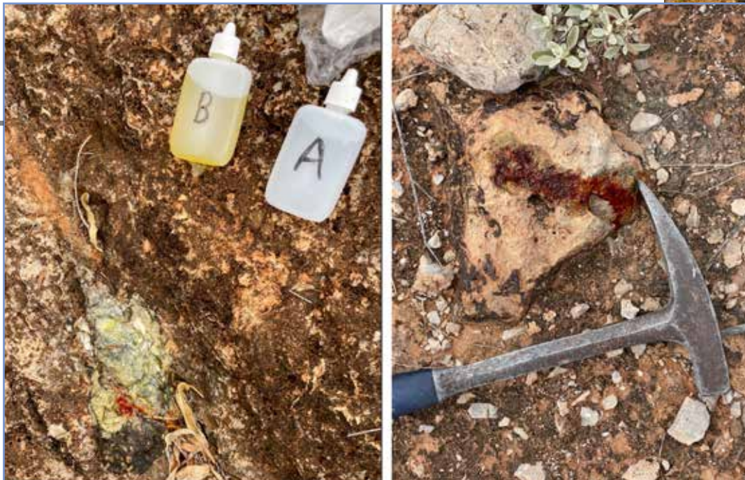
Figure 8: Examples of a positive (red) zinc-zap wet chemical test in the new area west of Linda.
