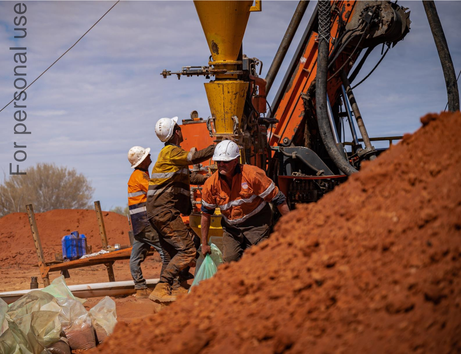
Figure 6: RC drilling underway at Aurora Tank during the financial year
