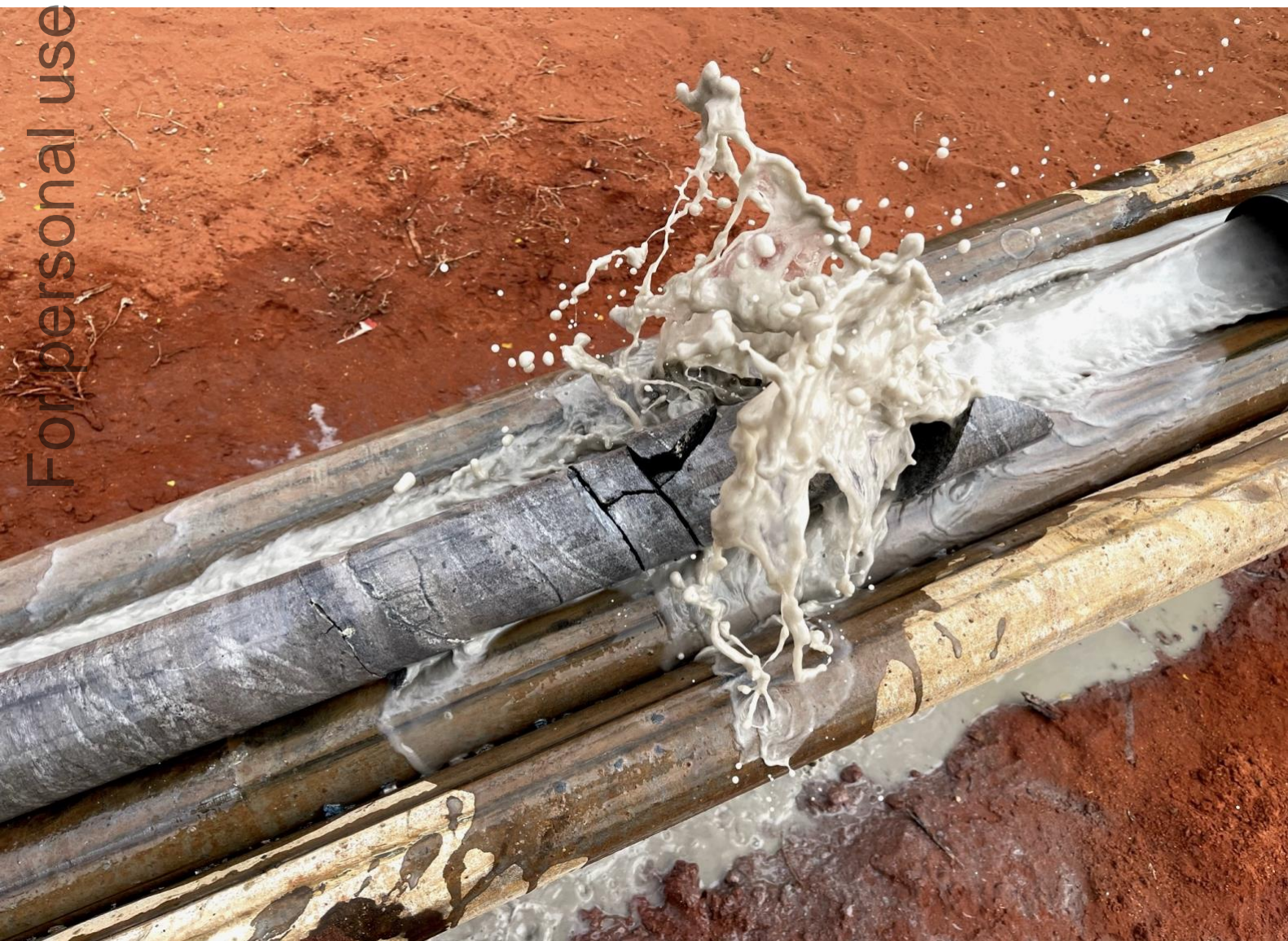
Figure 7: Diamond core being pumped out of the drilling rods at Aurora Tank (May 2023)
