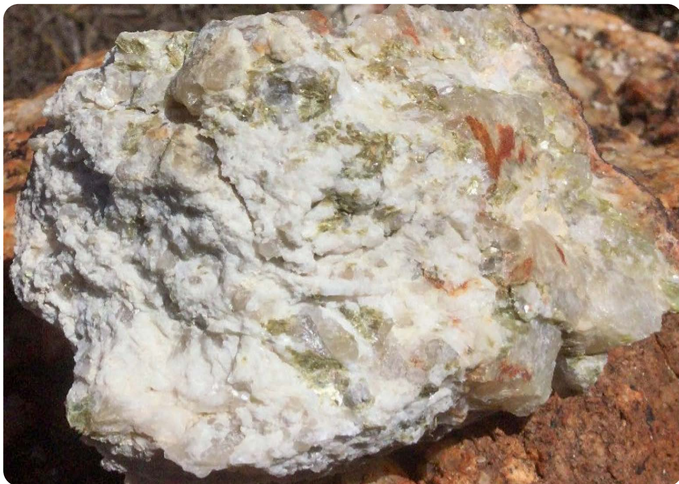
Micaceous Pegmatite rock chip sample MW2211_15 from the western margin of Orelia Target 1. Exhibited geochemical responses of LCT pegmatites. Assayed 2.7ppm Bi; 59ppm Li; 14ppm Be; 31ppm Cs; 61ppm Nb; 1055ppm Rb and 30 ppm Ta (See ASX Announcement 6 December 2022)
