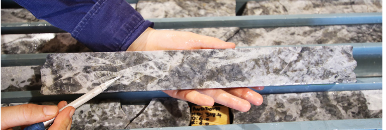
Figure 5: Coarse-bladed spodumene in quartz in hole ANDD0199. This sample returned 1.0m @ 1.52% \text{Li}_2\text{O} between 317m-318m
