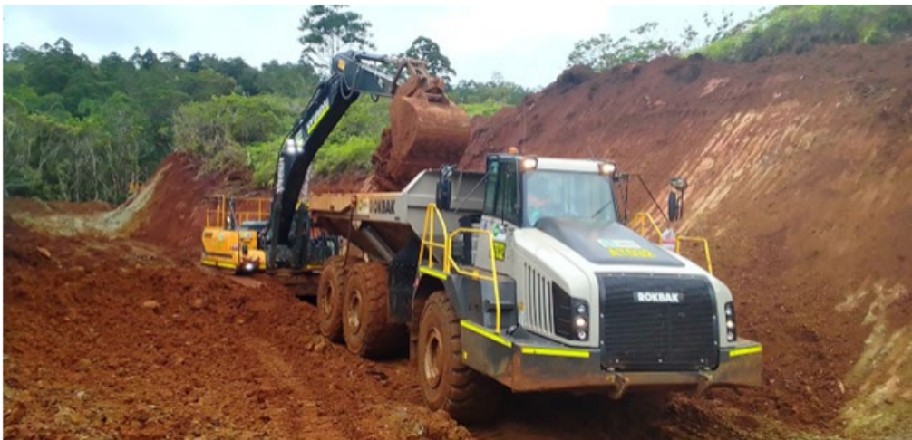
Removal of overburden in the first ore blocks for the mining of ore planned to commence in October 2023
