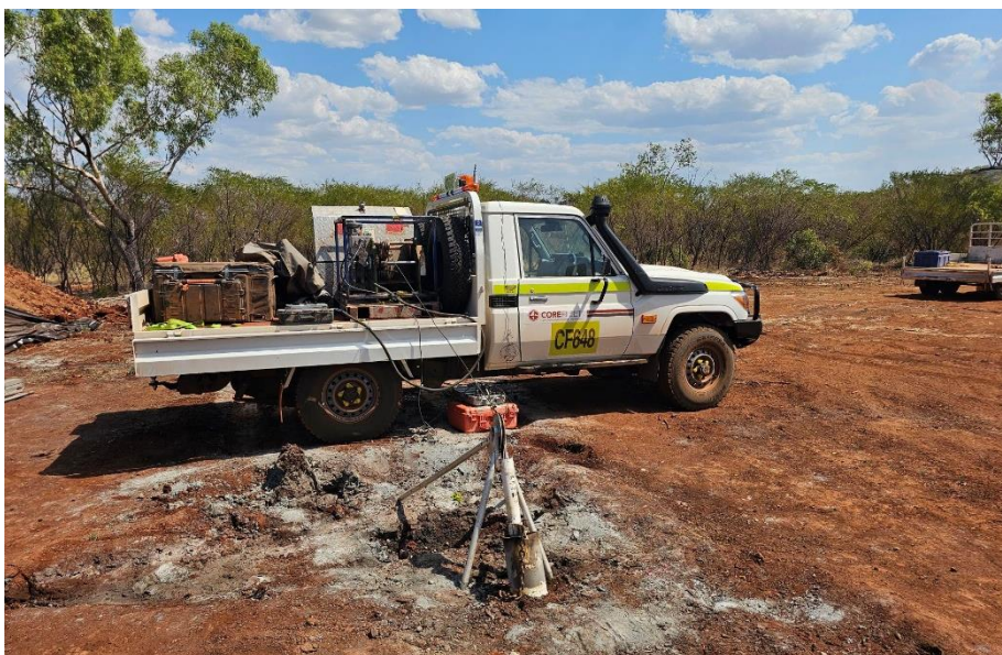
Figure 1. Downhole Electromagnetic Survey set up at BRDD001
