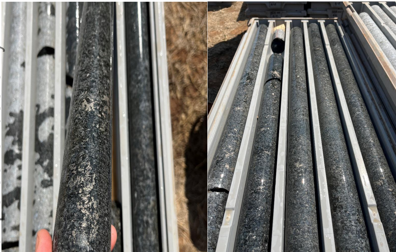
Figure 2. Photos showing examples disseminated and blebby sulphides in hole BRDD002. (Left) Blebby sulphides at 345m. (Right) Disseminated sulphides 338 – 342m Note core is NQ2 being 2 inches or 50mm in diameter
