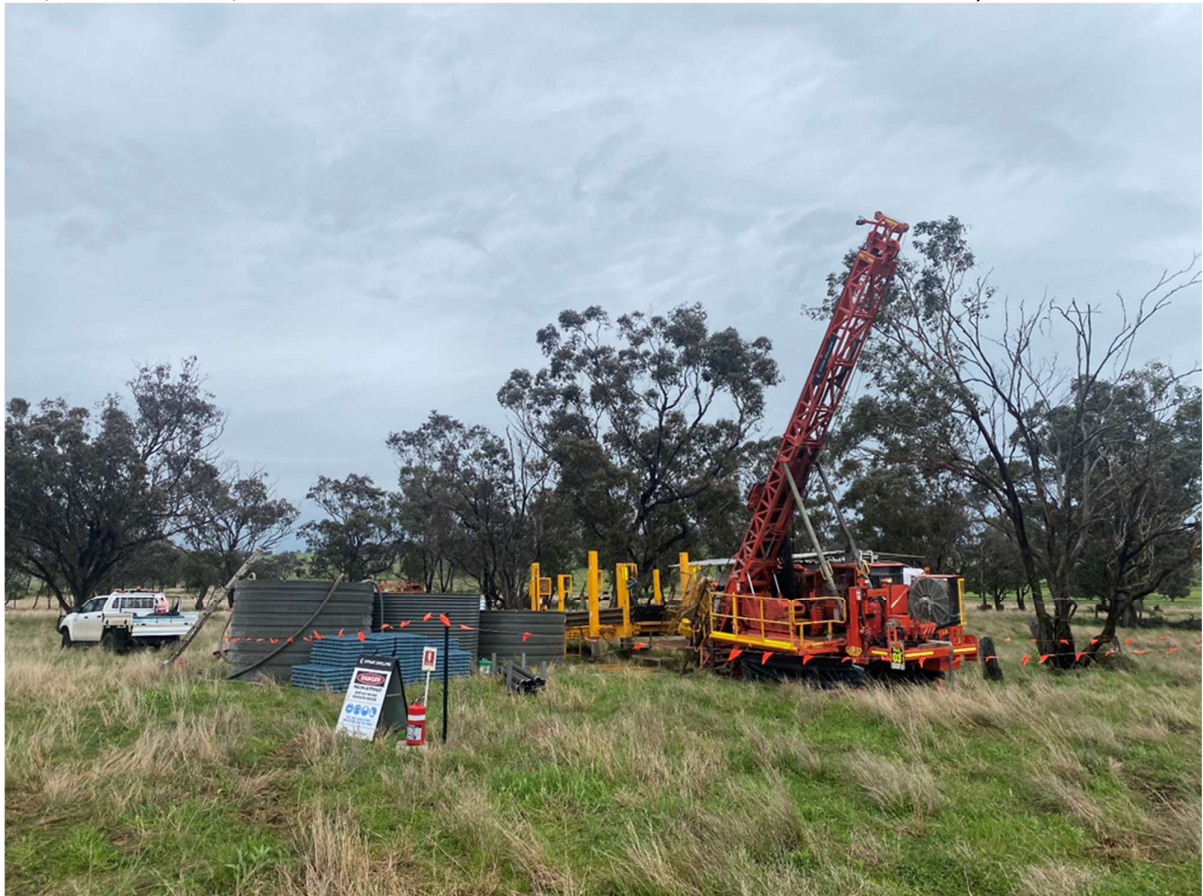
Figure 9 - Diamond core drilling 22BEDH011 at Boda East
