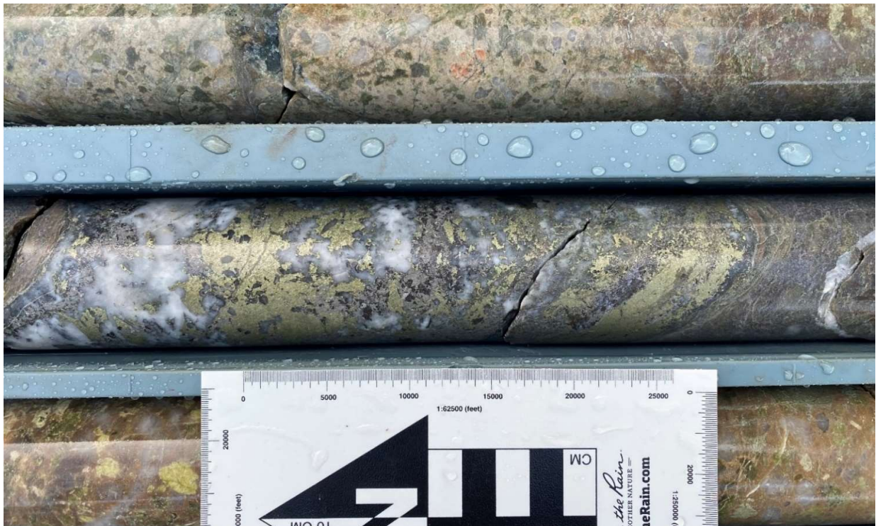
Figure 10 - High grade copper (1m @ 3.0% Cu from 173m) recently intersected in drill hole 22NGD108, forms within a mineralised interval reporting 19m @ 0.3 g/t Au from 171m including 1m @ 3.5g/t Au from 181m (22NGD108).
