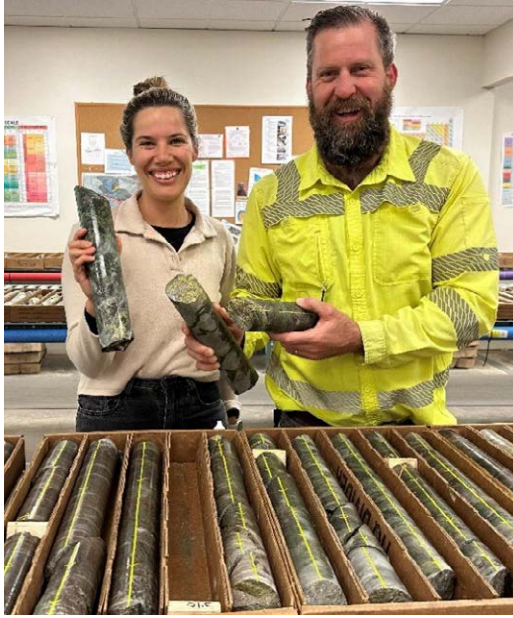
Chalcopyrite mineralisation in WTU-23-06 from 100m to 105.2m, within an 11.4m thick zone grading 2.29% Cu, 16.45g/t Ag and 0.14g/t Au. Bree Ivory (Corporate Affairs Manager) and Brian Paull (Director of Exploration) holding core from WTU-23-06
