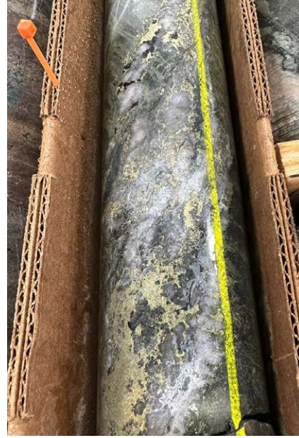
Chalcopyrite mineralisation in WTU-23-06 from 100m to 105.2m, within an 11.4m thick zone grading 2.29% Cu, 16.45g/t Ag and 0.14g/t Au. Bree Ivory (Corporate Affairs Manager) and Brian Paull (Director of Exploration) holding core from WTU-23-06
