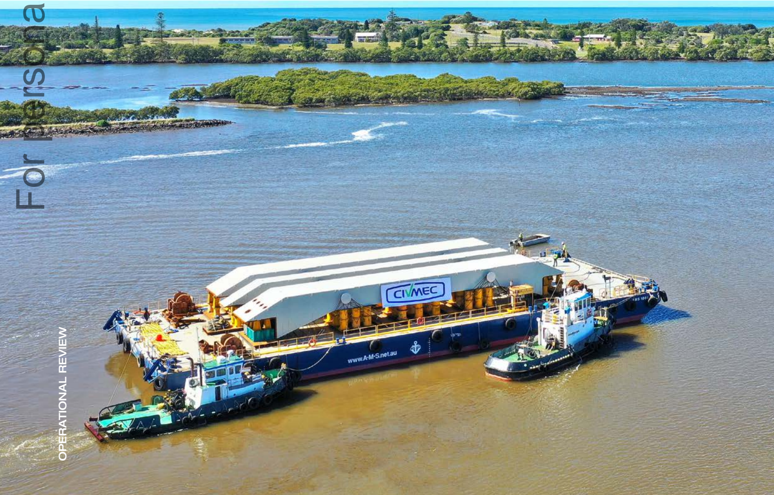
SABR Project dogbone ballast beams en route to Hay Point
