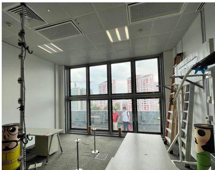
Second Generation ClearVuePV vision glass testing IGU's and spandrel panel units (above the glazing) installed and being prepared for commencement of BCA testing.
