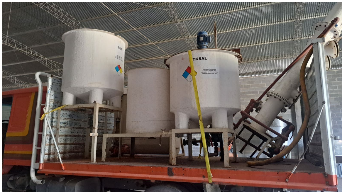
Figure 1 – Plant mixing tanks and columns being relocated to the new Pursuit Lithium Facility in Salta, Argentina.
