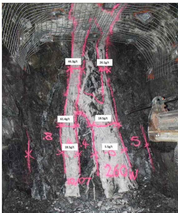
Pictures: Ok Underground 260W OD1 Face 13 showing annotated grades (Left) 215E OD2 Face 5 (Right).
