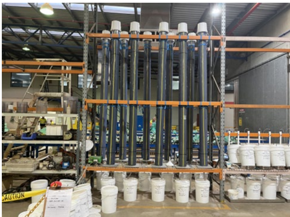
Plate 3 – Column Leach test work towards optimising gold recovery on Apollo Hill mineralised samples.
