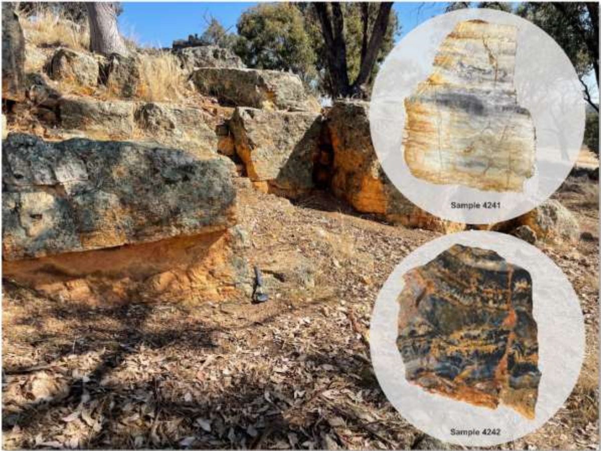
FIGURE 3: SINTER OUTCROP AT THE BRECCIA SINTER PROSPECT, AND INSERTS SHOWING SINTER RELATED LITHOLOGY SAMPLE 4241 OF THE BRECCIA SINTER PROSPECT AND SAMPLE 4242 FROM THE QUARRY PROSPECT. SAMPLES SHOW DOMINANT LIGHT AND DARK GREY CHALCIDONIC-QUARTZ BANDING WITH YELLOW TO LIGHT BROWN OXIDES AFTER POSSIBLE IRON-CARBONATE.
