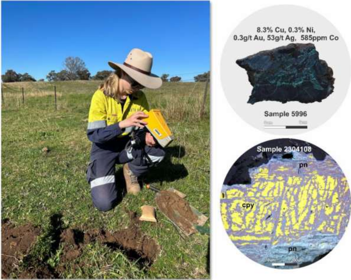
FIGURE 9: EARTH AI FIELD TEAM CONDUCTING SOIL SAMPLING AT FONTENOY (LEFT), AND ROCK SAMPLE 5996 (TOP RIGHT), AND NICKEL SULPHIDES (PN - PENTLANDITE), COPPER SULPHIDES (CPY - CHALCOPYRITE) CONFIRMED IN SERPENTINITE/GABBRO THROUGH SEM AND PETROGRAPHIC ANALYSIS (BOTTOM RIGHT).
