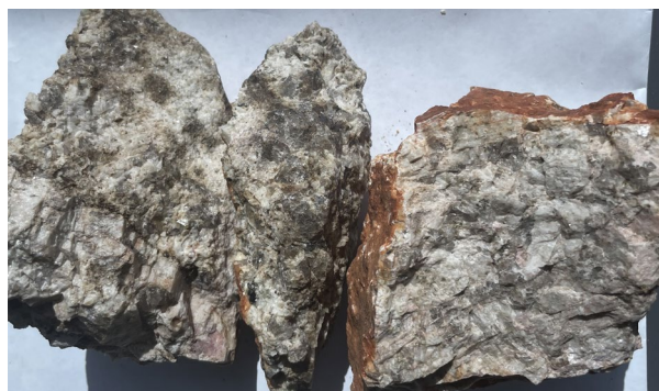
Figure 4: Sample 198116 showing the highest fractionation and highest readings of Ta_2O_5 (33.3ppm) and Nb_2O_5 (109ppm).
