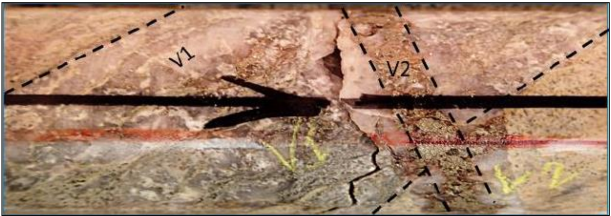
Figure 9: Thin pyrite-rich V2a vein crosscutting obliquely a quartz-carbonate-pyrite V1 vein, MSDD007, 260 m.
