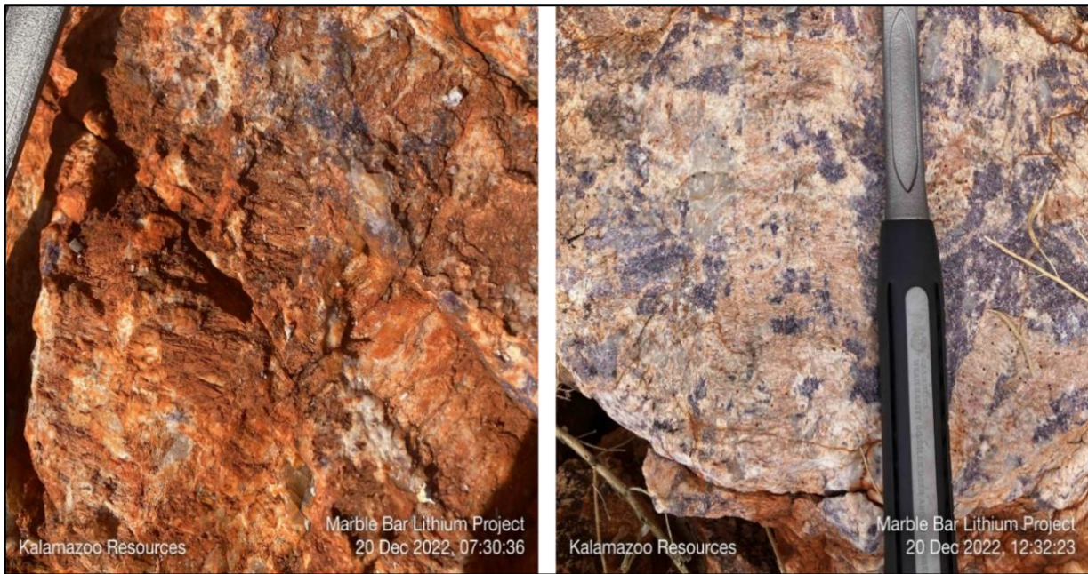
Figure 12: Example photos of spodumene (pale pink-white, coarse elongated striated mineral) and lepidolite (purple) mineralised pegmatite dyke in E45/5970, Marble Bar Lithium Project, East Pilbara WA. Note these photos correspond to rock chip sample MBLR212 which assayed 2.8% Li 2 O (see Table 3). Scale of view is ~40cm.
