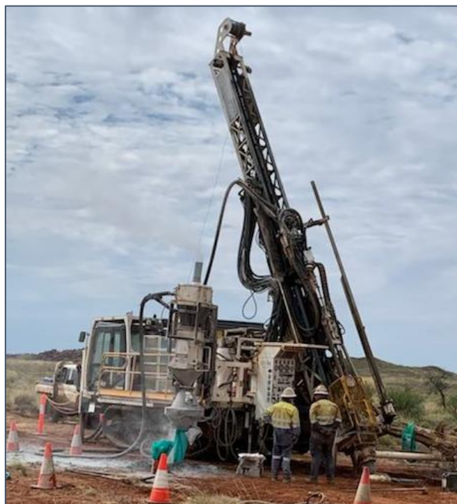
Figure 5: Maiden RC Drilling Program at Mallina West
