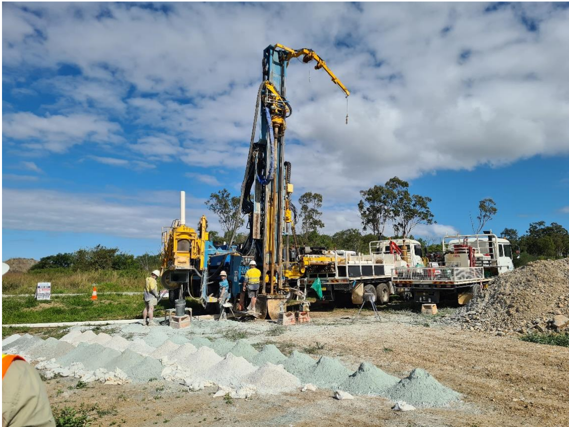
Figure 8: QMines' RC drill rig and support vehicles drilling at the Mt Chalmers project.
