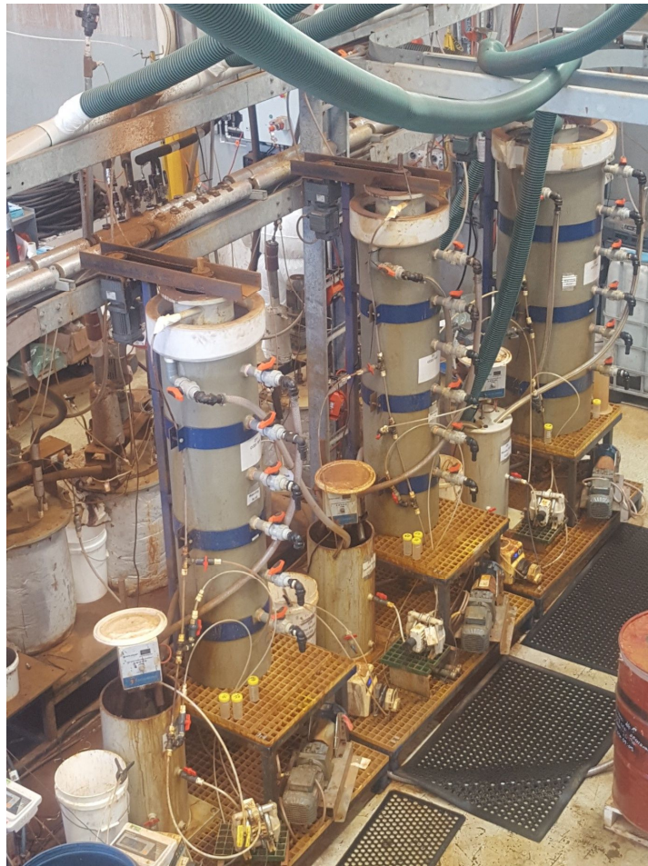
Figure 5. Counter Current Decantation piloting
