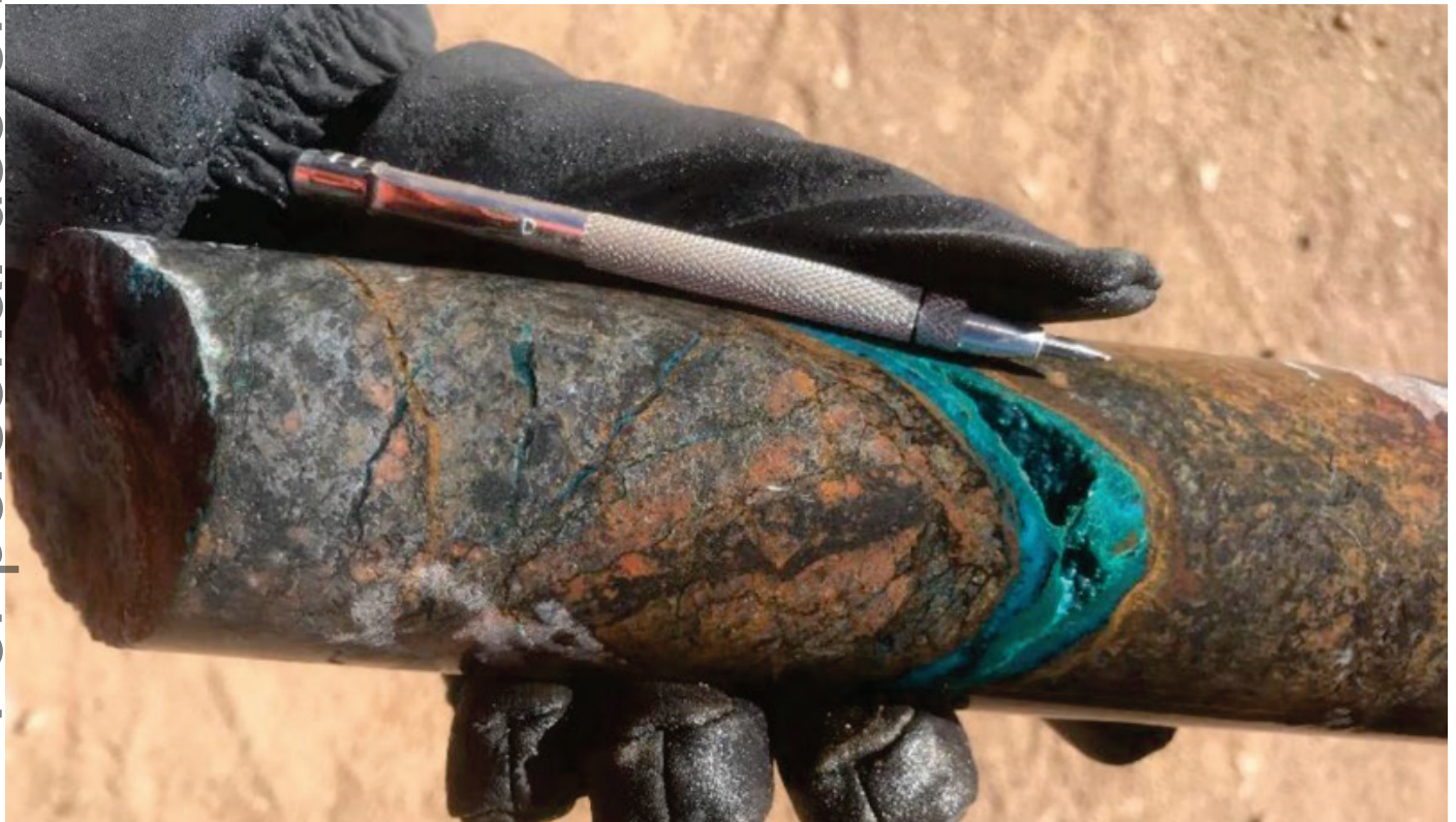
Figure 11: Drill core from hole PNSI22-001 at 89m showing quartz-malachite-azurite-chrysocolla veins
