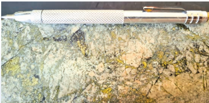
MET025 (179.15m depth down-hole) – vein-hosted and disseminated chalcopyrite and pyrite in tourmaline breccia. Interval graded 2.1% CuEq (1.9% Cu, 0.3% Au, 129ppm Mo).
