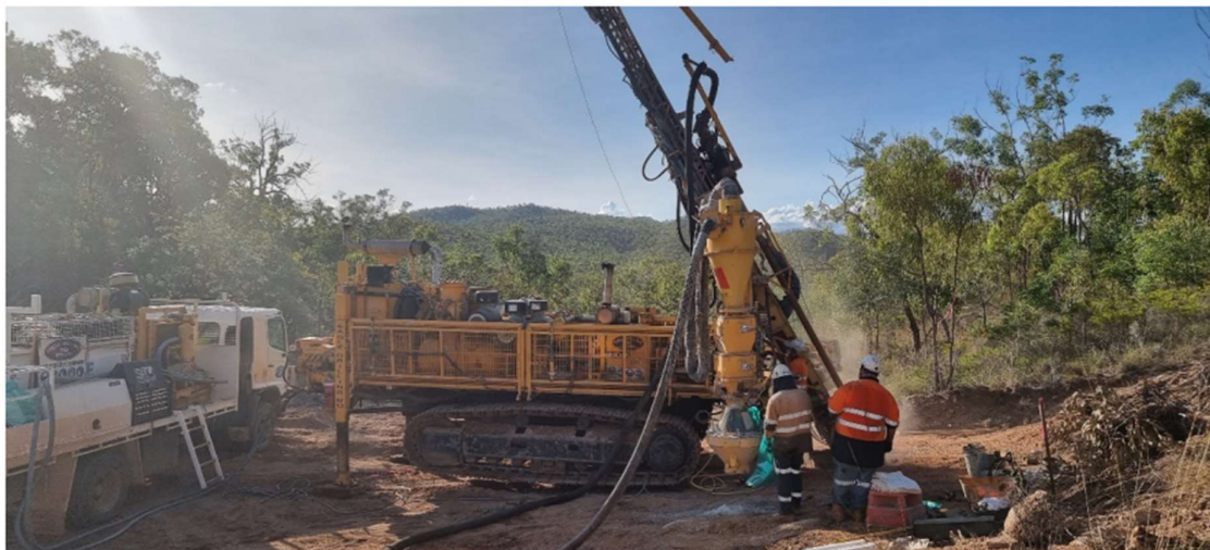
Photo 1: RC drilling at Adelaide Prospect
