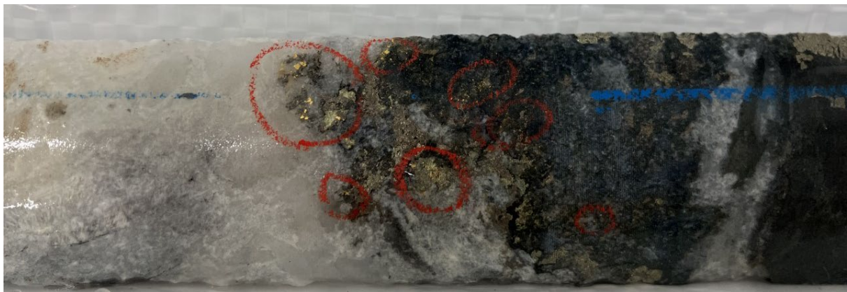
Image 1: Photograph of the quartz vein margin of the intersection in hole AUDD0333 grading 0.4m @ 1,020g/t gold. Drill core size is NQ.
