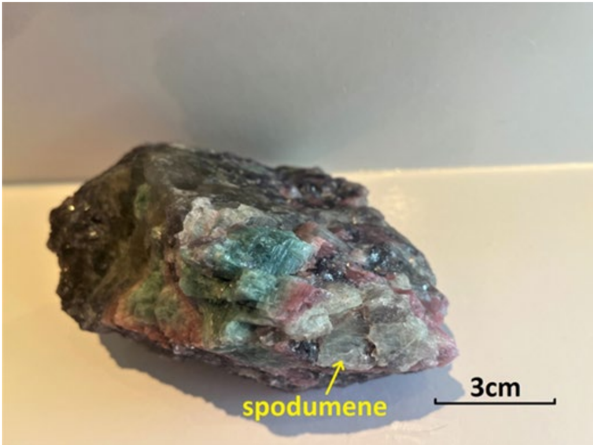
Figure 9: Specimen of spodumene-bearing rock from Muvero East. Rock comprised of approximately 50% lepidolite, 35% quartz, 10% elbaite (pink and green) and 5% spodumene.
