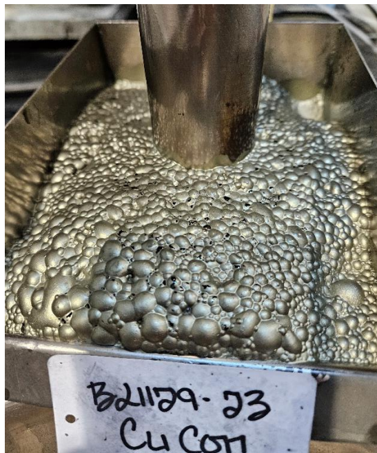
Flotation of copper during initial locked cycle test work
