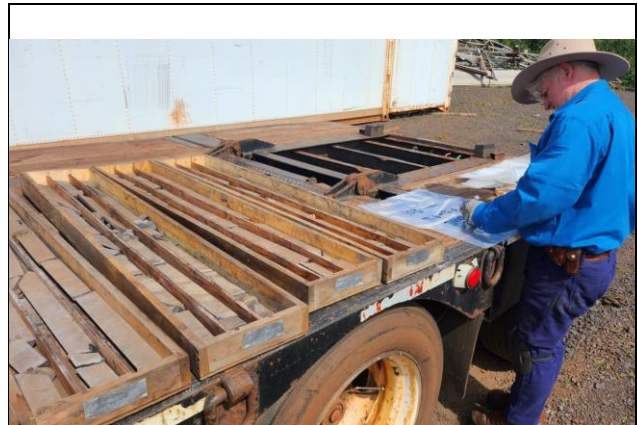
Consulting Geologist and Mining Engineer selecting and logging representative taconite
