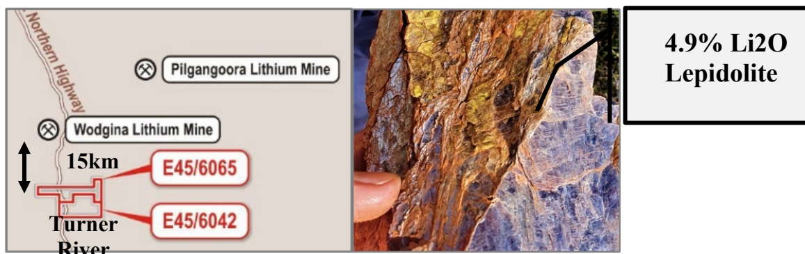
Figure 1: Location map of QXR's Turner River project mineral exploration licences relative to large Pilbara lithium mines, and photo of weathered lepidolite in rock samples from the drilling area shown in Figure 1.
