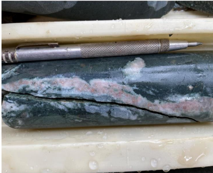
Photo 2. 22RRD-03 159.20m-160.80m depth contains dense silica+carbonate veins, up to 1-3% native copper
