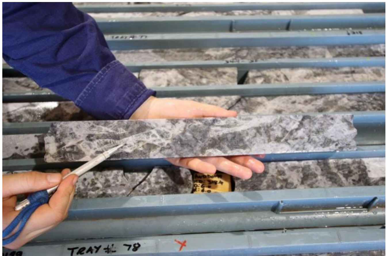
Figure 5: Coarse-bladed spodumene in quartz in hole ANDD0199. This sample returned 1.0m @ 1.52% Li 2 O between 317m-318m
