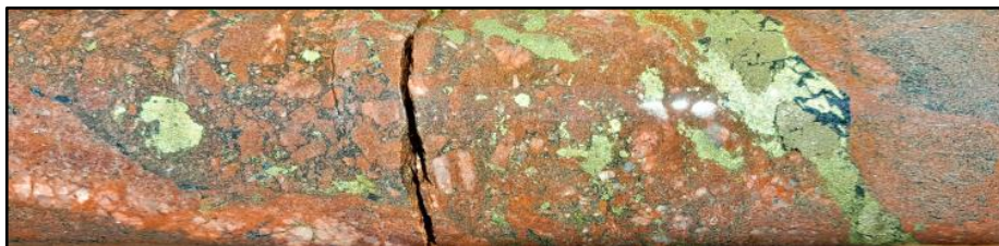
Figure 10: HWDD08 1040.7m 2cm massive chalcopyrite >pyrite-minor magnetite vein, with 5cm magnetite-chalcopyrite-pyrite breccia in footwall.
