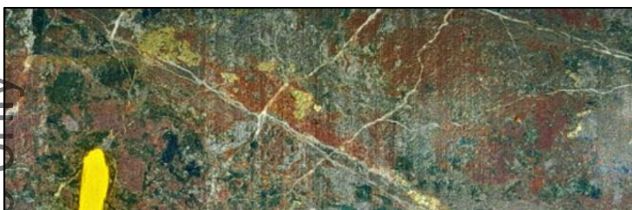
Figure 7: HWDD07 1157m. Vein and disseminated chalcopyrite in altered mafic intrusive in the footwall of the upper Bluebush Fault.
