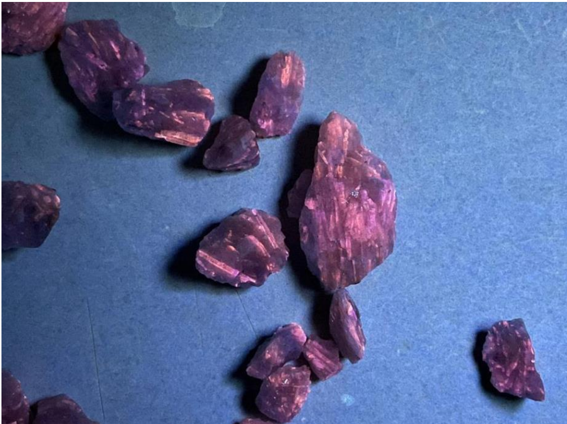
Figure 12: Spodumene crystals in HYRC006 (162-163m) under 250nm ultraviolet light (1m @ 0.47% Li 2 O)
