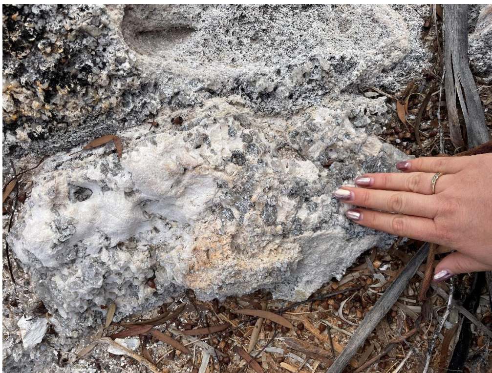
Figure 4 – Example of the intensely weathered pegmatitic rocks from the Lake Johnston Project
