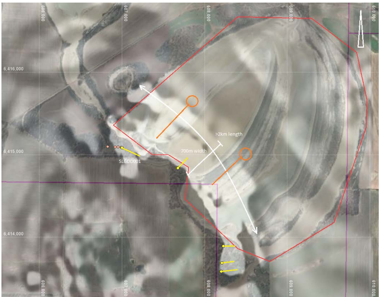
Figure 10: Plan view of 1VD magnetic signature representing the ultramafic sequence overlain by aerial photography highlighting the salt lake, with Reserve 18455 (Lot 225568) highlighted in red. Sultan's 2022 aircore collars are marked in orange, and previous diamond drilling traces in yellow, with recent SLGDD001 named. Orange circles and traces indicate provisional drilling collar positions to test the layered intrusion correctly.
