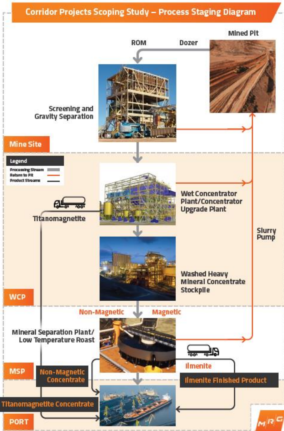
Figure 5: Scoping Study Process Staging Flowsheet – Corridor Sands Project (Koko Massava, Nhacutse and Poiombo Deposits).
