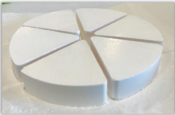
Sintered HPA feed material from the HPA First Project
