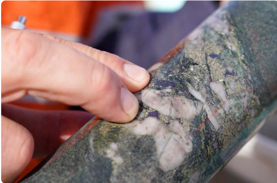
Figure 3. Quartz vein (15cm) with bornite (blue), pyrite and minor chalcopyrite at 221.2m
