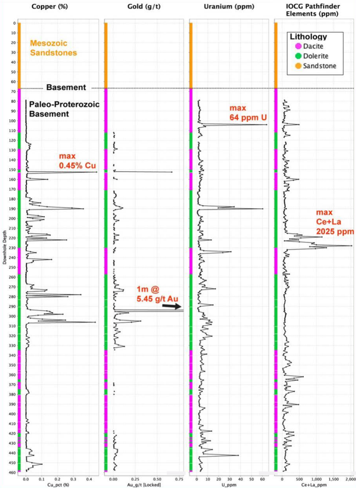
Figure 4. Strip-log of drill hole 23PK01 demonstrating typical element association of Cu, Au, U, Ce and La with an IOCG-style mineral system. (CUS ASX Release 24-7-2023)
