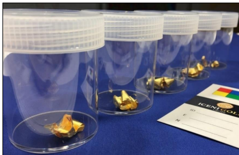
Figure 8: Gold recovered after fire assaying the high-grade Christmas Gift vein samples; these samples returned 18,207g/t Au, 18,179g/t Au, 16,776g/t Au, 16,659g/t Au and 14,780g/t Au (in ASX release dated 13 July 2023).
