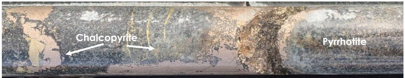
Figure 17. Massive sulphides in TMDD0001, chalcopyrite, pyrrhotite and pyrite observed, 841m depth 7,13 .
