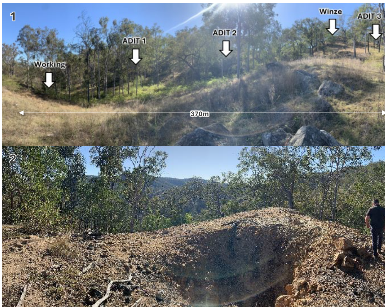
Figure 4. Old Copper Workings, 1. Historical copper workings of the mine from the early 1900's, includes three adits into the hill, and one winze for hauling copper ore out of the mine. 2. Photograph of the historical copper mine winze (1920's), with view down to old adits which extend into the hill over a strike of 370m. This is just one of eight old mines identified. Rock chips samples were collected from old mine workings as well as veins in subcrop-outcrop, August 2023.
