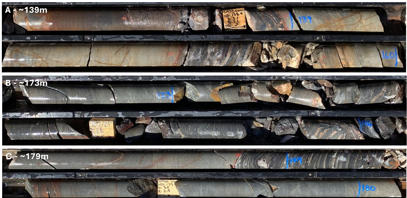
Figure 16. Diamond core photographs of the iron-rich sediments of the Dead Bullock Formation (DBF). A) At approximately 139m, folded iron-rich sediments of the DBF. B) Folded siltstone and shale units of the DBF at ~173m, with multiple folding and shearing events overprinted, with k-feldspar alteration. C) Sediments of the DBF, with increased pyrite and quartz veining 9 .
