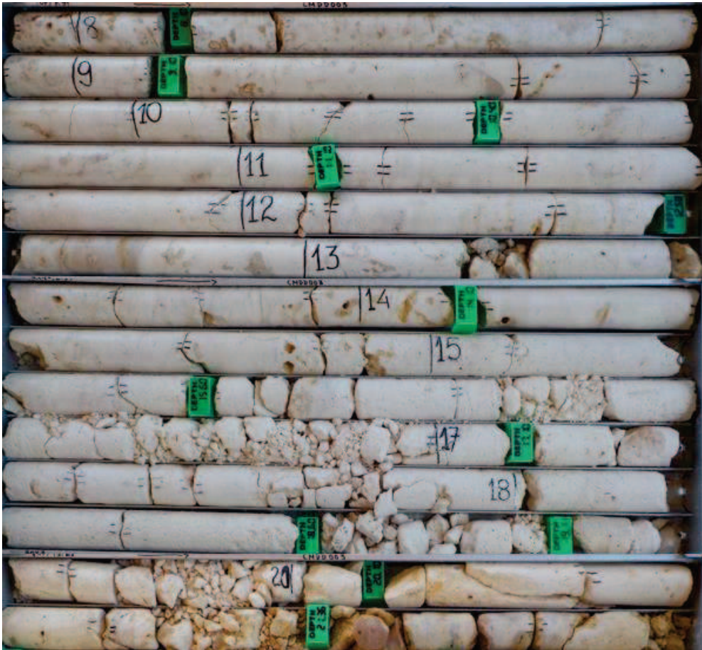
Fig 4: High purity Limestone (CMDD003) from 8.00 to 21.30m with weighted average 98.04% CaCO 3
