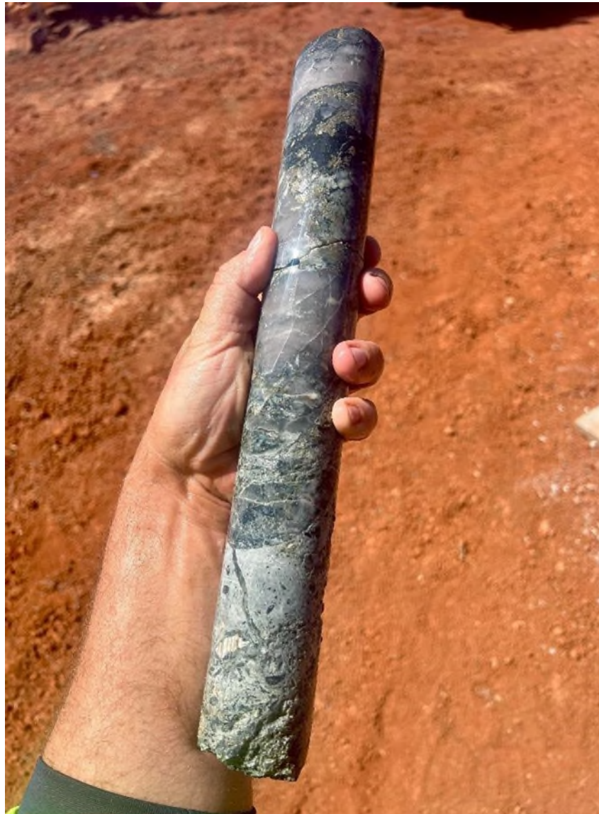
Figure 14: Shear zone with silica flooding and minor sulphides
