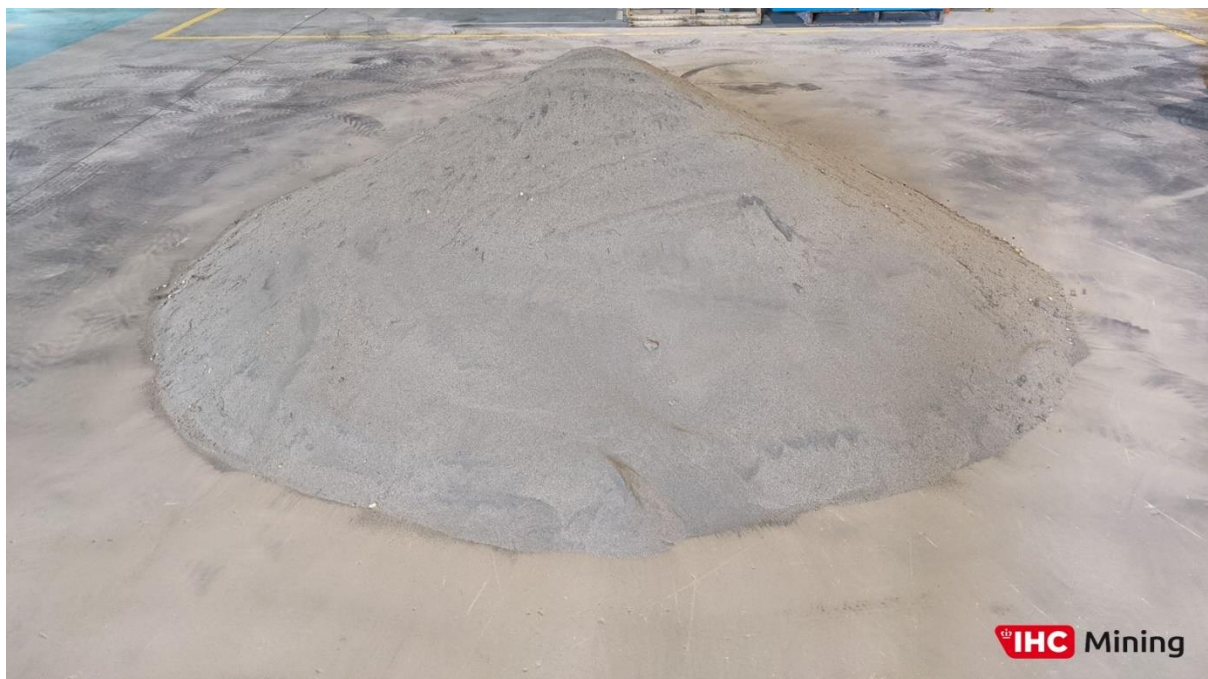
Plate 1 – “Run of mine” magnetite bearing industrial sand sample prepared for pilot plant processing
