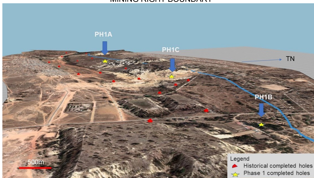
IMAGE 5: PLAN VIEW OF THE BIRD REEF CENTRAL AND WEST EXPLORATION TARGET AREA, WITHIN THE WBP’S MINING RIGHT BOUNDARY
